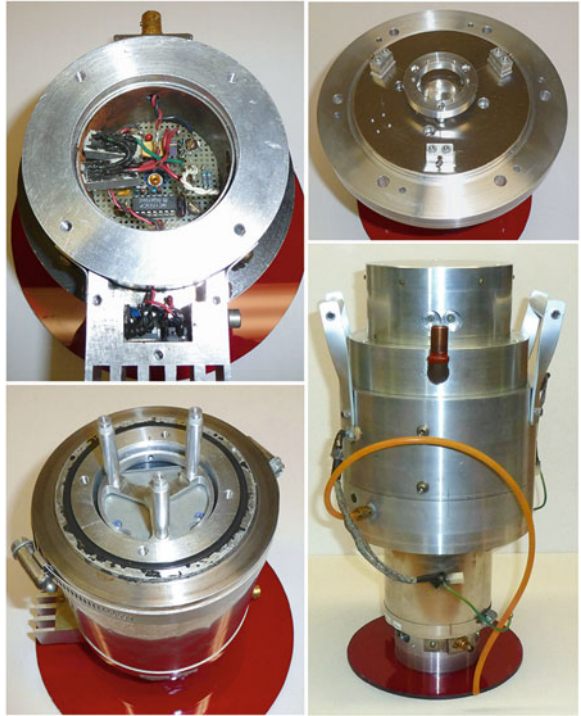
Fig. 4.2 Views of the early weight/thrust sensor. In the upper left panel are the Wheatstone bridge electronics in their chamber mounted directly below the U-80 sensor chamber. In the lower left panel the U-80 sensor is shown mounted in its concentric aluminum and steel chamber. An aluminum ring that supports three rods that pass through the base plate of the main test chamber is shown attached to the end of the shaft of the U-80 sensor. In the upper right panel the main chamber base plate is added, along with the support ring tensioned by fine steel wires. In the lower right panel the entire test chamber is shown fully assembled
