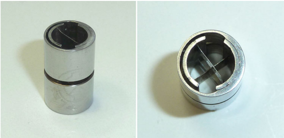
Fig. 5.1 Two views of a C-flex flexural bearing of the type used in the USC/ARC style thrust balance. The crossed steel leaves attached to the two halves of the tubular shell provide a restoring torque when the upper and lower halves are rotated with respect to each other
