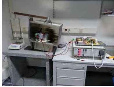
Setup with Box on Knife-Edge Balance
