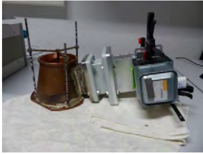
Thruster Model with Magnetron
