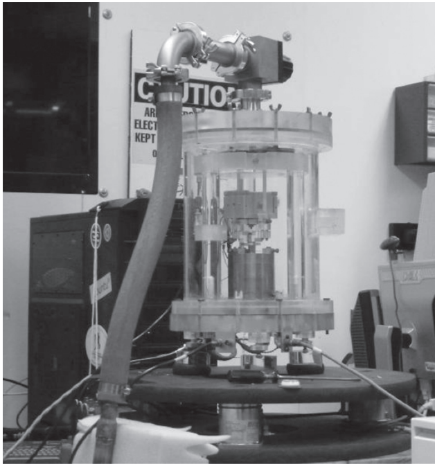
Fig. 7 Vacuum chamber with rubber isolation feet on top of a platform with 3 pneumatic vibration isolation stabilizers. A long copper pipe ran from the vacuum pump to the chamber in order to reduce vibrational noise from the pump.
