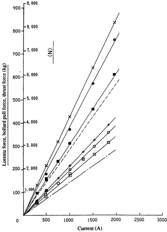
**Fig. 13 Results of Bollard Pull Force Measurement**
