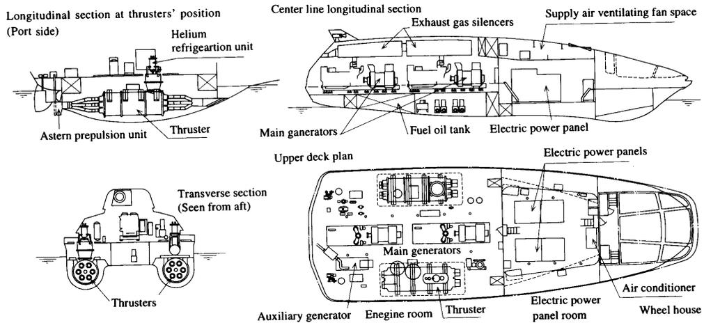
**Fig. 2 General Arrangement of "YAMATO 1"**
