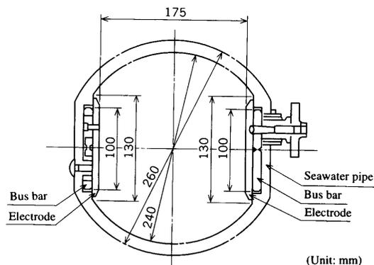
**Fig. 5 Cross Section of Seawater Pipe**
