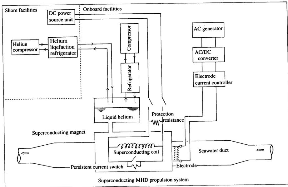
**Fig. 3 Outline Diagram of Propulsion System "YAMATO 1"**
